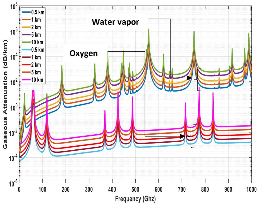
Figure 4. Gaseous attenuation in Lagos (South West) at different heights.
