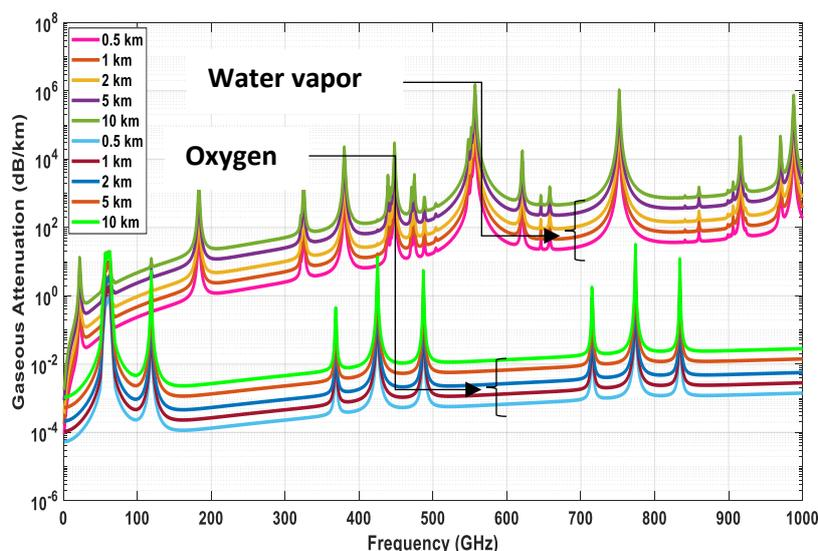
Figure 2. Gaseous attenuation in Abuja (North Central) at deferent heights
