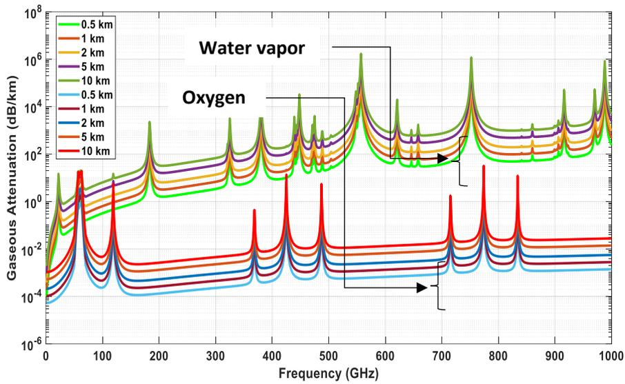
Figure 5. Gaseous attenuation in Portharcourt (South South) at different heights
