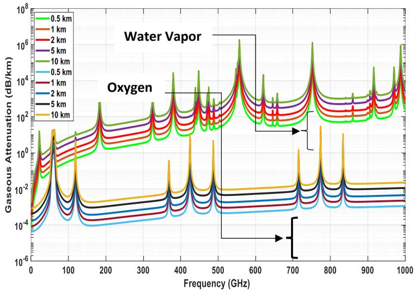
Figure 6. Gaseous attenuation in Enugu (South East) at different heights
