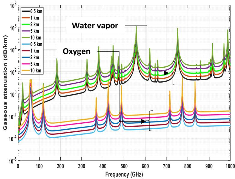
Figure 3. Gaseous attenuation in Bauchi (North East) at different heights
