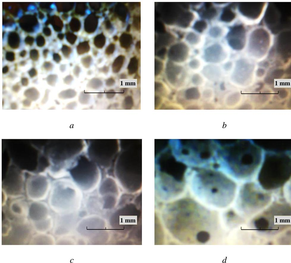
*Figure 4. Pictures of the microstructural configuration of the glass aggregate samples
