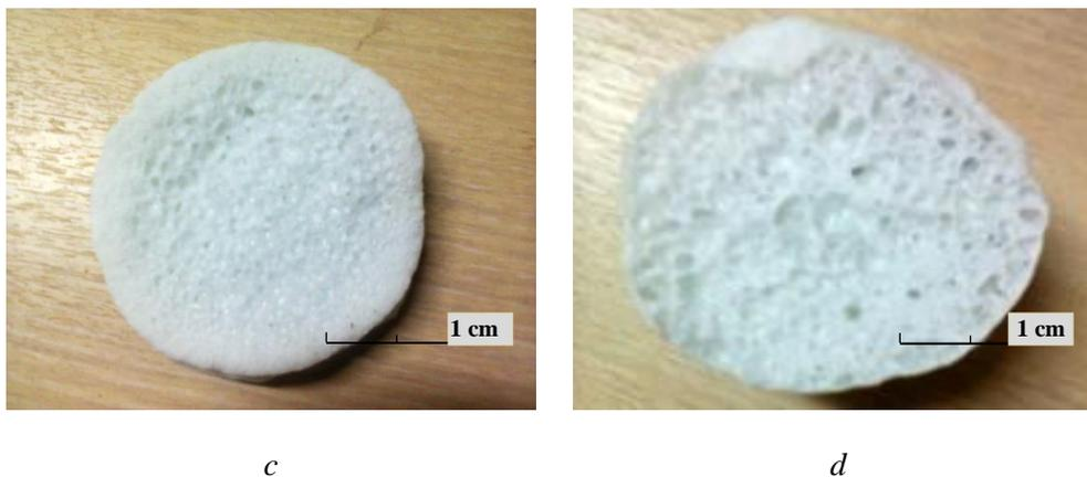
Figure 3. Section of sintered glass aggregate in form of pellet
