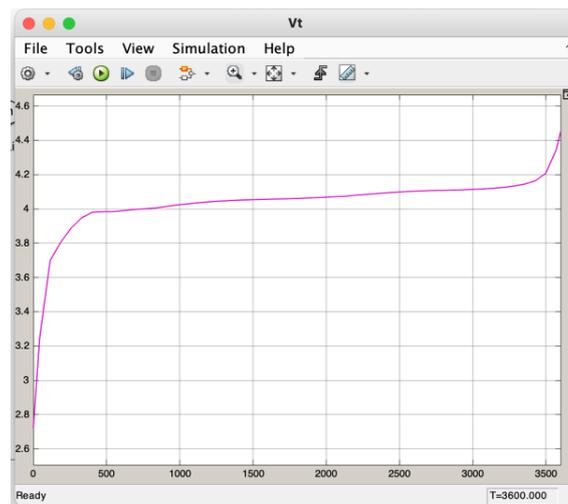
Figure 7. Terminal Voltage of 4V battery charged over 1hour (3600 Sec).
