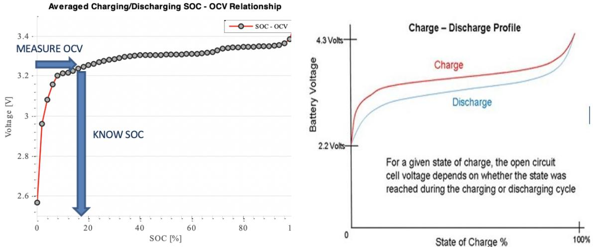
Figure 4. Charge and Discharge profile of a battery
