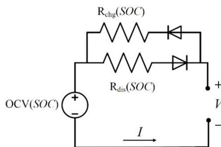
Figure 2. Electric Circuit of battery
