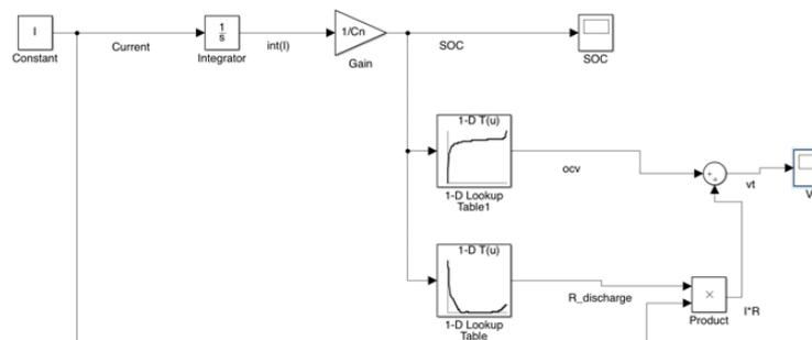
Figure 8. Simulink model representing equation 1 and equation 2.
